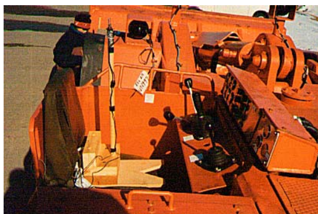
Figure 2: Seat point indicator with light filament located in the LHD operator's seat.
